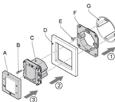
1. Attach the wall frame (F) to mounting box (G). Use the correct screws (E).
