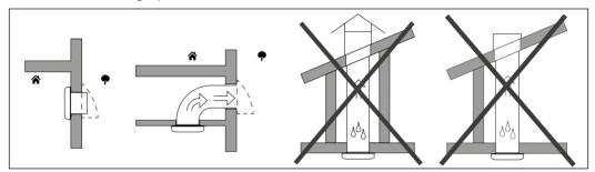
The unit can be installed in bathroom zone 1 (except for the power cable from above), provided that the installation and wiring are in accordance with IEC 60364-7-701 (current version) and in accordance with the national standards of the country of installation.
