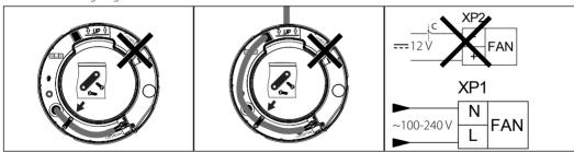
Remove the plugs before connecting to the XP2 connector.
