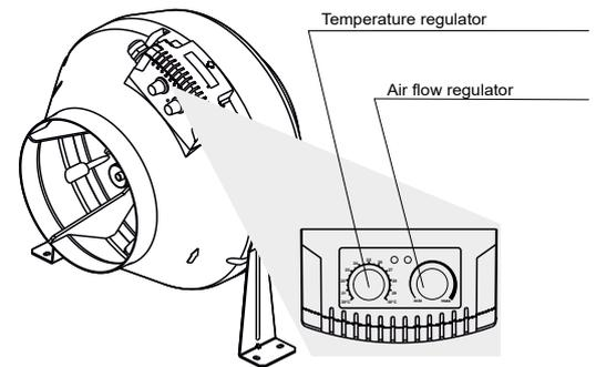
The **VK ... ECP** fan is equipped with a built-in smooth speed controller that enables switching the fan on/off, smoothly adjusting the rotation speed (air flow) in the range from minimum to maximum speed.
