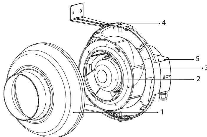
The fan is equipped with a single-phase electronically commutated (EC) motor with an external rotor equipped with a centrifugal impeller.
