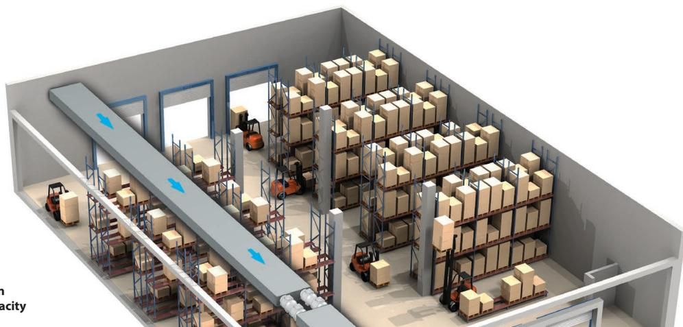
parallel mounting of the fans in storage room increases air capacity
