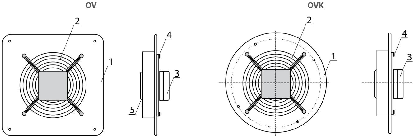
The **OV1** and **OVK1** fans consist of a casing 1 made of polymer-coated stainless steel with a square (**OV1**) or round (**OVK1**) flange, to which the grille 2 is fastened with bolts 4. The motor and impeller 5 are mounted on a bracket inside the casing. The fans are equipped with a terminal box with a cable for remote connection.
