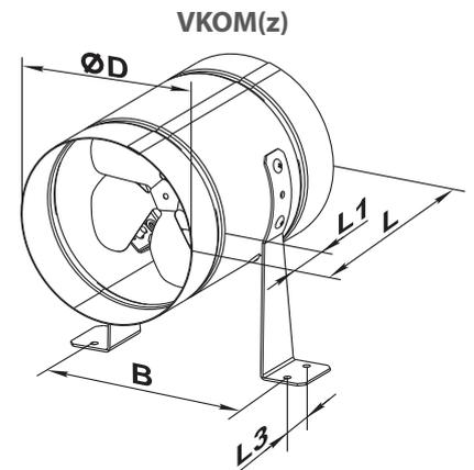
The **VKOM(z)** fans are equipped with **RM(z)** (polymer-coated steel, galvanised steel) reducers for connection to 150 mm, 200 mm and 250 mm air ducts.
