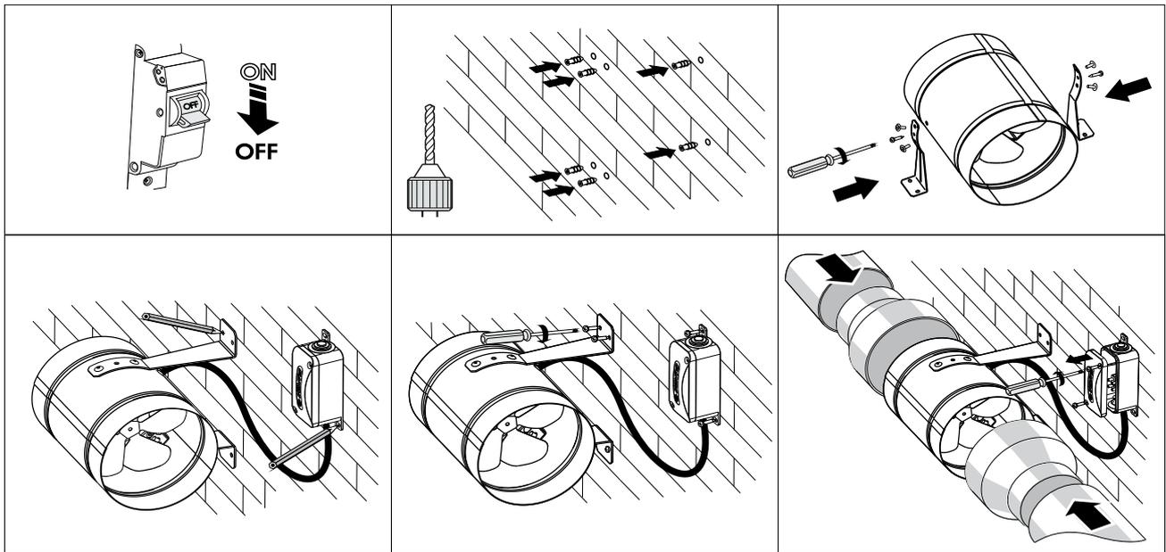
2. Note: the mounting bracket fixing point on the fan casing must be selected so that the screws do not interfere with the free rotation of the impeller.
