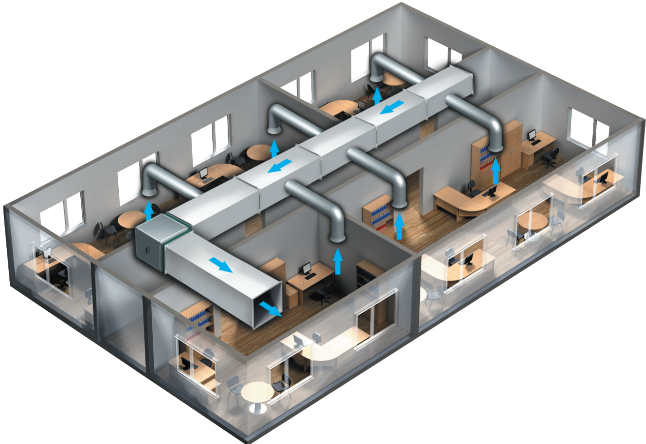
VS EC fan office ventilation example
